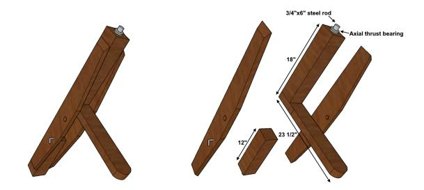
Once the holes are drilled, screw one end of the 23.5" long  $2^{\circ}x4^{\circ}$  to the 18" piece of 4"x4", at the opposite end to the one holding the steel rod.
