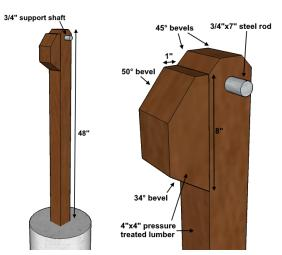
Once the adjustment block is installed, drill a  $\frac{3}{4}$ " diameter hole through the centre of the east-west faces of the support post, approx. 1  $\frac{3}{4}$ " from the top of the post to the centre of the hole, then install a  $\frac{3}{4}$ "x7" steel rod in the hole and leave an equal portion projecting from each side to receive the strongback later.
